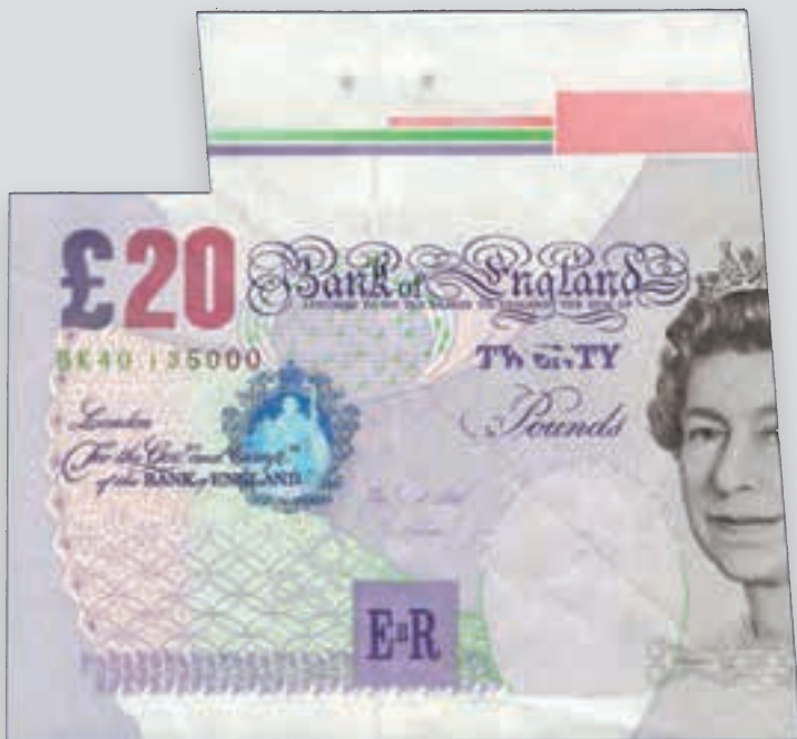
31 ERROR: Bank of England, Merlyn V. Lowther, £20, 1999, serial number BK40 135000, with a significant cutting error because of a fold in the paper during printing, resulting in extra paper along the top edge of the note, including colour bars, and the right hand side of the note being omitted, good extremely fine EPM B386 £200-£260
