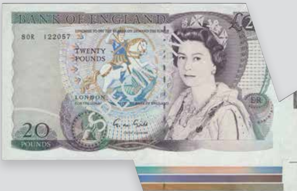
26 ERROR: Bank of England, George M. Gill, £20, 1988, serial number 80R 122057, with significant extra paper error, including colour bars, resulting from a double fold in the paper during printing, uncirculated and a spectacular error EPM B355 £200-£260
