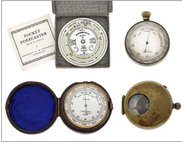
280 A pocket forecaster by Negretti & Zambra, in original box, a leather cased circular gilt pocket barometer retailed by Army & Navy Stores Ltd, London, and another similar, retailed by Reese, Portmadoc together with a pocket compass, first diameter 53mm.
