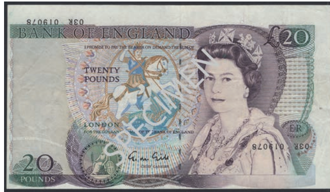
32 ERROR: Bank of England, George M. Gill, £20, 1 March 1988, serial number 03R 019078, with cutting error and upside-down serial numbers, presumably resulting from the note being printed correctly, but the sheet then being inserted upside-down into the cutting and numbering machine, very fine and extremely unusual EPM B355 £150-£200
